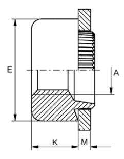
Female thread A = M3Height K = 3.0Outer diameter E = 8.0Plate thickness = 1.4 to 1.6
